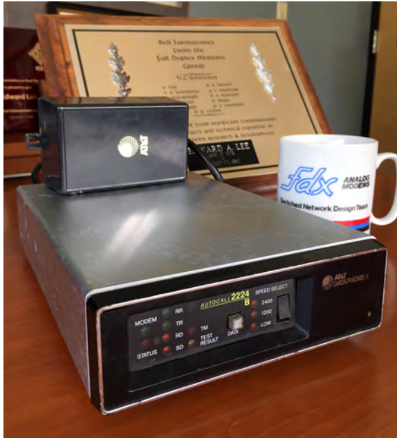
Figure 9.1: A vintage voiceband data modem, the first to be realized by software, designed by the author and colleagues at Bell Labs in the early 1980s.
