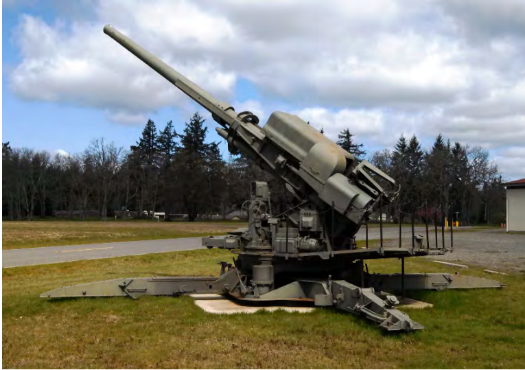
Figure 5.4: 120mm anti-aircraft gun, deployed near the end of World War II. These guns were automatically aimed using negative feedback by the M10 director system, which used information from a radar system, and the M4 gun computer. This gun is on display at the Washington National Guard Museum, located on Camp Murray in Washington State. Courtesy of the Washington National Guard State Historical Society.
