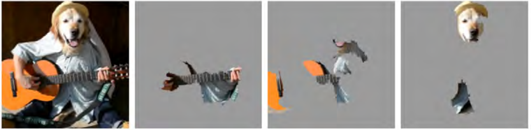
Figure 6.1: Explaining an image classification prediction made by Google’s Inception neural net by identifying the portions of the image that most influenced Inception to choose classes “electric guitar,” “acoustic guitar,” and “labrador” as the top three best matches. From Ribeiro, Singh, and Guestrin, (2016).
