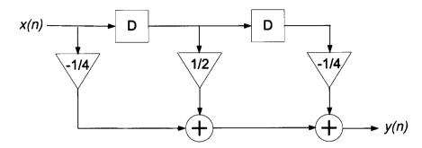
(a) Determine the linear, constant-coefficient difference equation governing the filter F.
