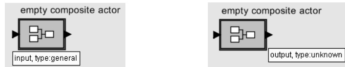
Figure 5.13 An empty transparent composite actor in Ptolemy II with input and output types displayed.
