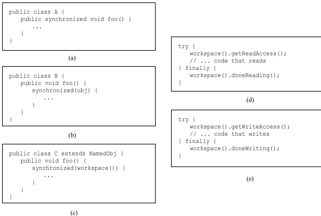
FIGURE 1.14. Using monitors for thread safety. The method used in Ptolemy II is in (d) and (e).
