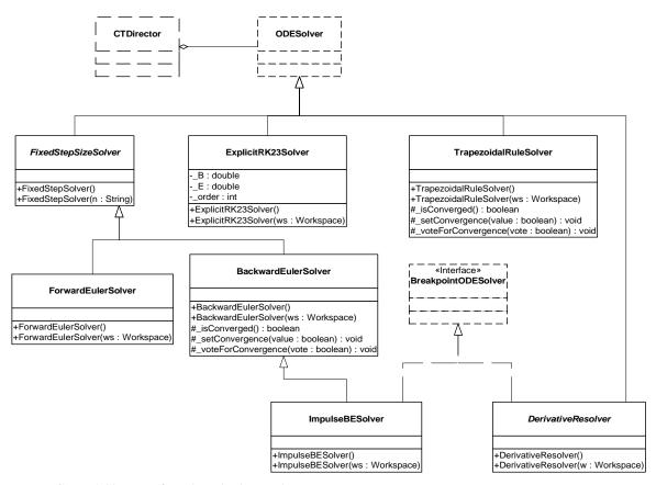
FIGURE 2.20. UML for ct.kernel.solver package.
