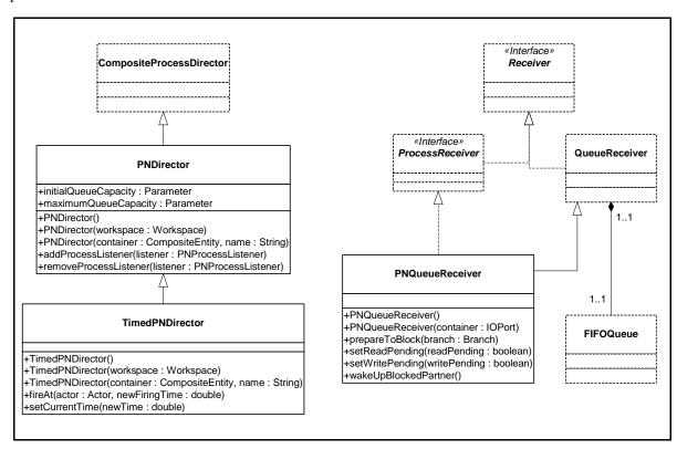
FIGURE 8.1. Static structure of the PN kernel.
