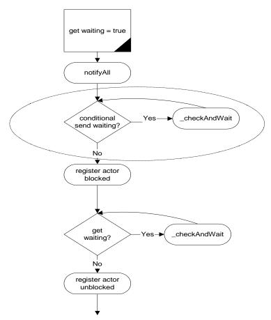
FIGURE 6.13. Modification of rendezvous algorithm, section 6.6.3, shown in ellipse.
