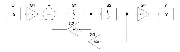
FIGURE 2.3. The block diagram for the example system.
