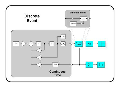
FIGURE 1.12. An example of heterogeneous and hierarchical composition. The CT subsystem and DE subsystem are inside an outermost DE system. This example is developed by Jie Liu [93].
