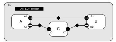
FIGURE 9.3. An example SDF model.
