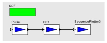
FIGURE 3.5. A model that plots the Fast Fourier Transform of a signal. Only one iteration must be executed to plot all 256 values of the FFT, since the FFT actor produces and consumes 256 tokens each firing.
