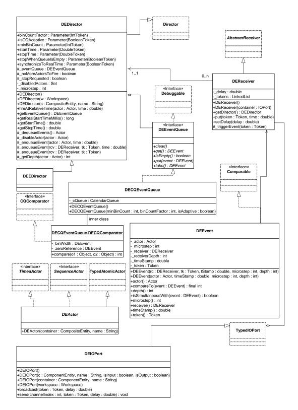
FIGURE 1.4. UML static structure diagram for the DE kernel package.
