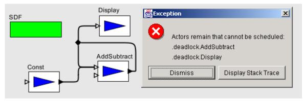
FIGURE 3.1. An SDF model that deadlocks.
