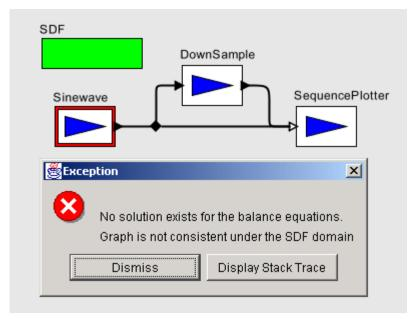
FIGURE 3.3. An SDF model with inconsistent rates.
