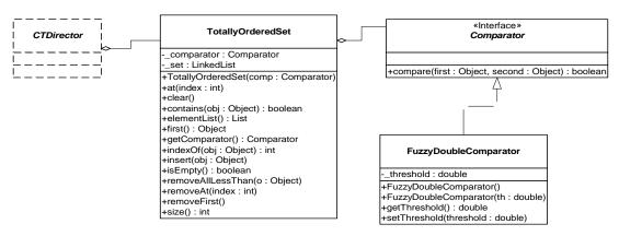
FIGURE 2.17. UML for ct.kernel.util package.
