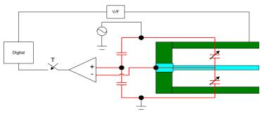
FIGURE 2.10. Micro-accelerator with digital feedback
