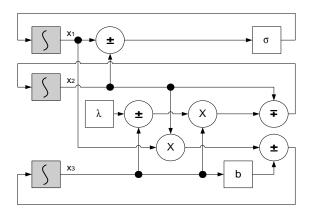
FIGURE 2.8. Block diagram for the Lorenz system.
