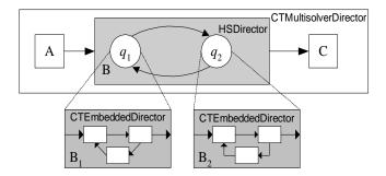
FIGURE 2.7. Hybrid system modeling.
