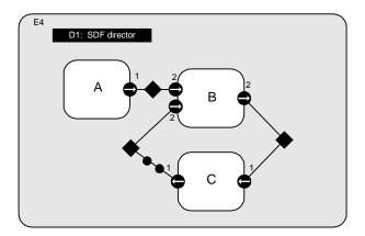
FIGURE 3.9. A consistent cyclic graph, properly annotated with delays. A one token delay is represented by a black circle. Actor C is responsible for setting the *tokenInitProduction* parameter on its output port, and creating the two tokens during initialization. This graph can be executed using the schedule A, A, B, C, C.
