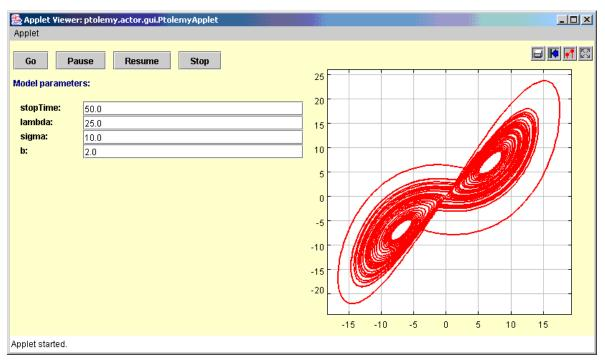
FIGURE 2.9. The simulation result of the Lorenz system.
