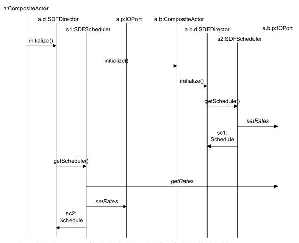
FIGURE 3.12. The sequence of method calls during scheduling of a hierarchical model.
