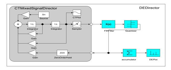
FIGURE 2.11. Block diagram for the micro-accelerator system.
