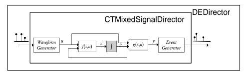
FIGURE 2.6. Embedding a CT component in a DE system.
