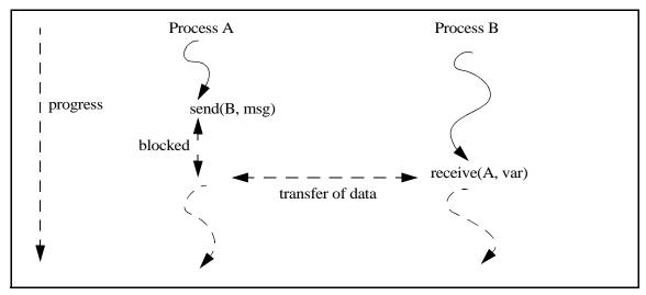
FIGURE 6.1. Illustrating how processes block waiting to rendezvous
