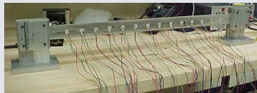
Simple beam vibration control
