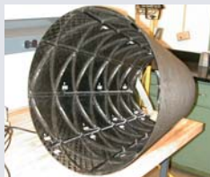
Complex structural acoustic control (launch vehicle payload fairing)
