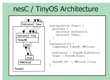
galsC extends nesC (the language used to specify TinyOS programs) to provide a GALS programming model that separates the rates of control of the system — the reactive part and the computational part — via asynchrony. galsC programs have minimal overhead, are easy to write and allow reuse of software components.
