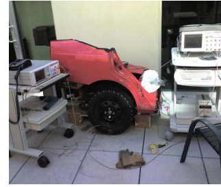
Fig. 6. Channel measurement setup.
