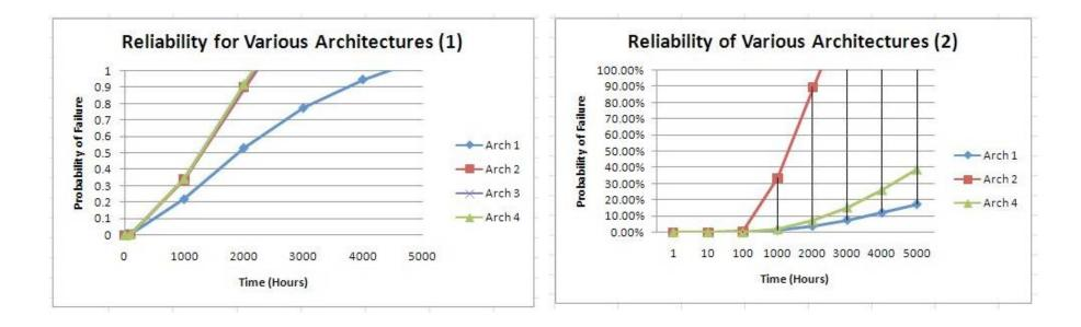
Reliability of various architectures from using initial sensor failure rate estimates (1) and by improving sensor failure rate estimates (2) based on basic event sensitivity results
