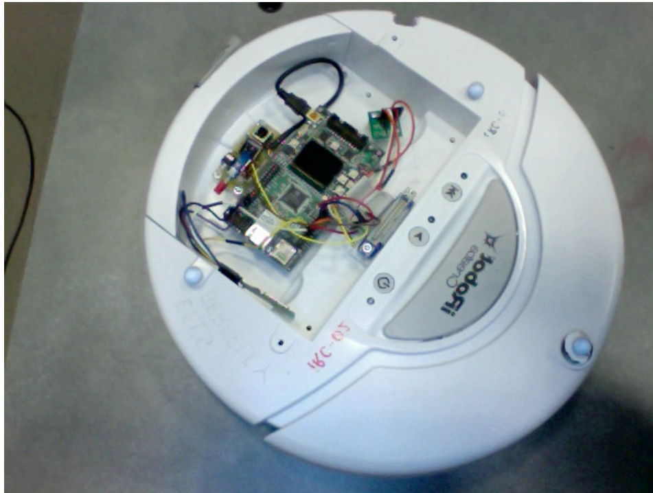
Fig.11. iRobot with 3 Reflective Markers
