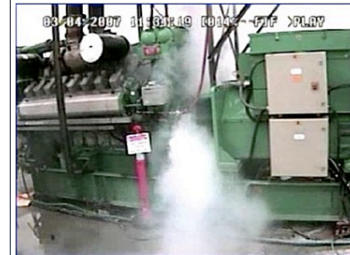
In this image from video released by the Department of Homeland Security, smoke pours from an expensive electrical turbine during a March 4, 2007, demonstration by the Idaho National Laboratory, which was simulating a hacker attack against the U.S. electrical grid. (AP Photo/Dept. of Homeland Security)
