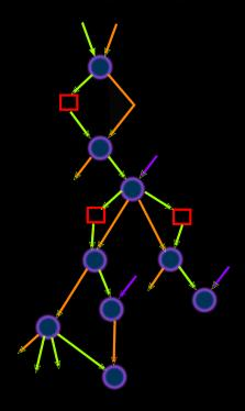
Here, an OEG can be given for a fragment of behavior associated with the actions in the configuration example. Orange arrows are control dependencies, green arrows are communication, and purple arrows are initialization. Red boxes are allocation events.
