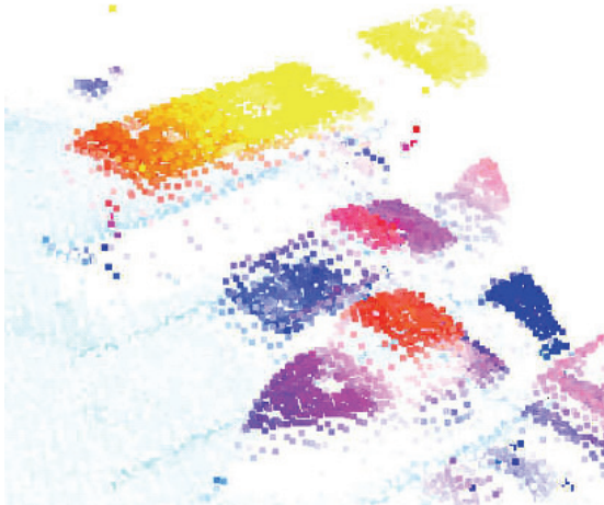
Figure 17: Vehicles detected at a >100m range using the flash lidar. The camera was mounted above the vehicles.
