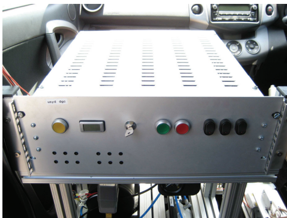
Figure 10: Main power/control box. The yellow (left) button indicates DISABLED mode, the green (just right of the key) RUN mode, the red (left of the three switches) PAUSE mode. The three switches to the right independently provide power to the individual actuators. The system is disabled without the key, and voltage to the system is displayed on the LED.
