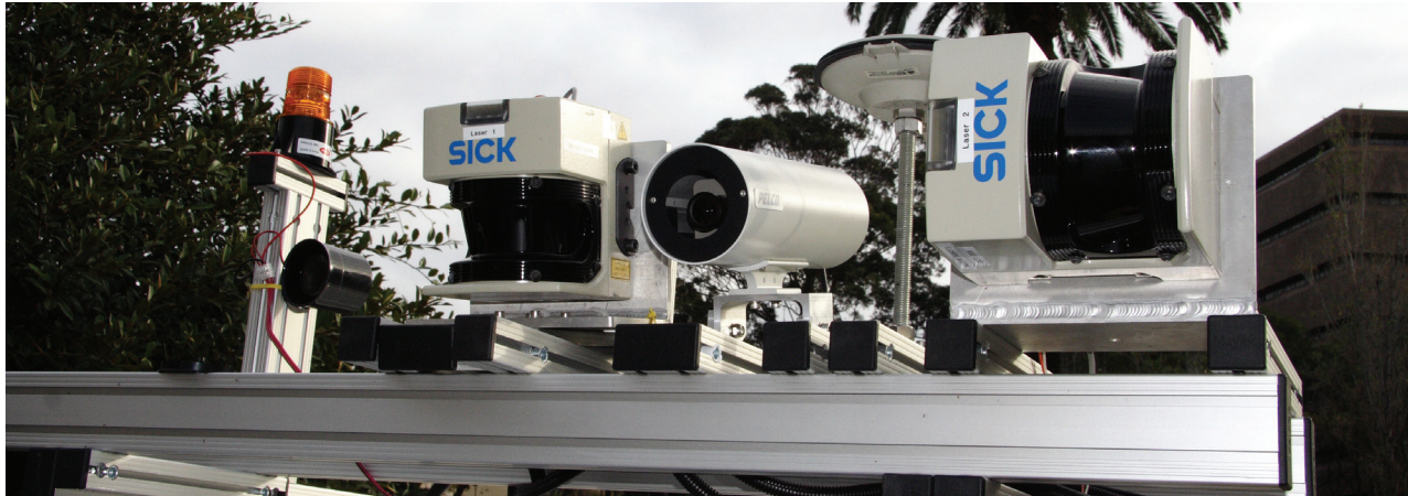
Figure 11: Current sensor suite – SICK lasers, INS, and camera.
