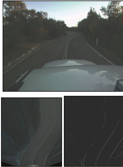
Figure 19: a) original image, b) IPM image, c) detected lane marking segments
