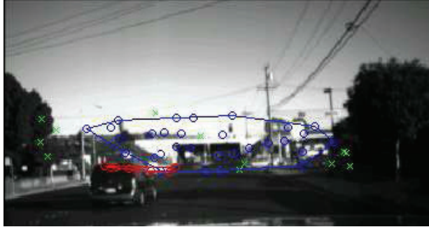
Figure 15. Being passed by another vehicle. The blue region is the largest labeled independently-moving object, and the red areas are other labeled independently-moving objects. The green points are unlabeled.
