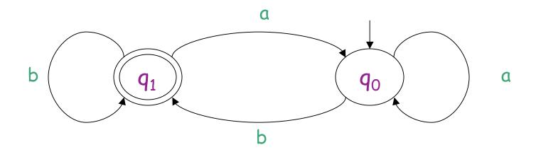
finite words: the run ends in an accepting state L(A)=(a+b)\*b
