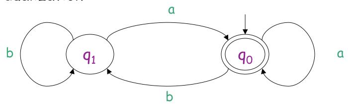
finite words: the run ends in an accepting state L(A)=(a+b)\*b  $L(\tilde{A})=\epsilon+(a+b)*a=(a+b)*$
