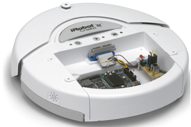
Figure 2: Early prototype of the Cal Climber cyber-physical system. The latest Cal Climber consists of an iRobot Create, a National Instruments Single-Board RIO (sbRIO), and an Analog Devices accelerometer.
