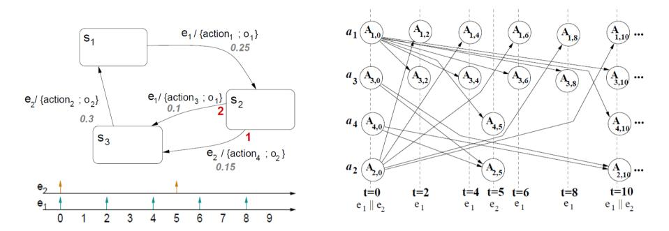
The true task graph model can be computed considering the time (in the hyperperiod) when actions can occur (WCETs and interarrival edges omitted).
