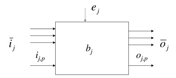
Stateflow (or state machine) blocks react to a set of events  $e_{j,v}$ , derived from signals (generated at each rising or falling edge).
