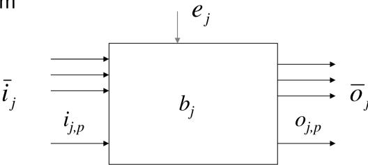
• At each  $e_j$  the block computes its out update and state update functions, updating the values on its output signals
