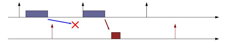
the system response or reaction must be completed before the next system event
