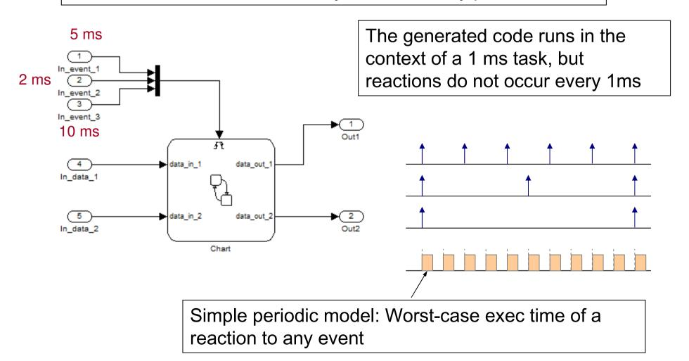
the system response or reaction must be completed before the next system event – if we abstract from the model and only look at the task code model, the analysis can be very pessimistic
