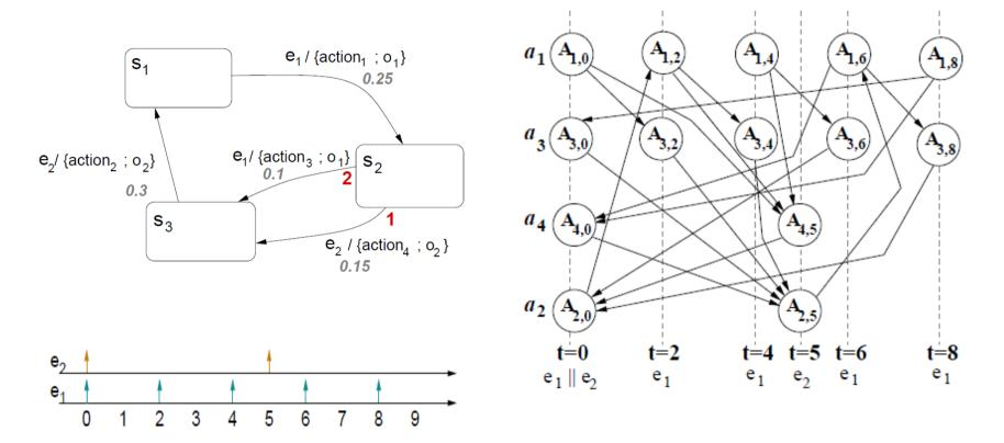
The digraph model can be simplified by removing the edges that are not critical to the schedulability analysis, and by folding vertices by exploiting the periodic pattern of the event arrivals in the hyperperiod.
