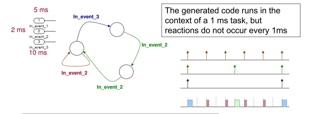
Even a multiframe model should account for state dependencies in the evaluation of the worst case execution time of each frame – need to build the right demand bound function
