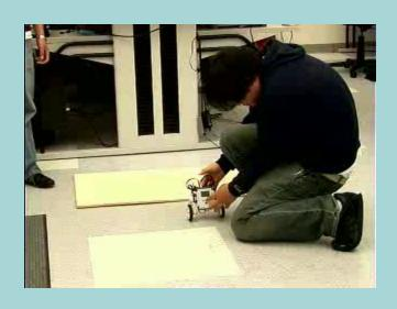
One of the five project teams in 2008 developed a balancing robot inspired by the Segway. They used a Nintendo Wiimote as a controller communicating with a PC running LabVIEW, communicating with a Lego Mindstorm NXT, which they programmed in C.
