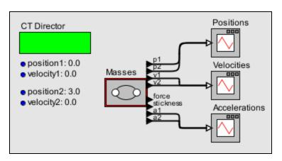
In the signals at the right, the velocities and accelerations proceed through a sequence of values at the times of the collisions and separations.
