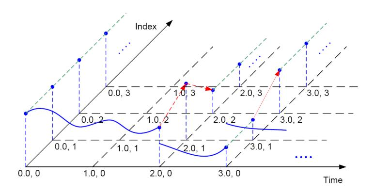
The red arrows indicate value changes between tags, which correspond to discontinuities. Signals are continuous from the left *and* continuous from the right at points of discontinuity.
