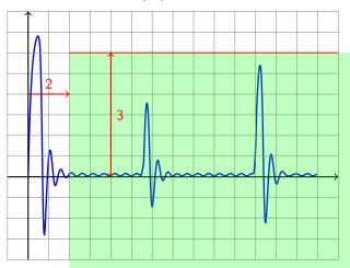
"Between 2s and 6s the signal is never above 2"  $\varphi := \text{ alw}_{[2,6]} \ \ (x[t] < 2)$
