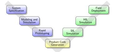
The model-based design (MBD) V design process.
