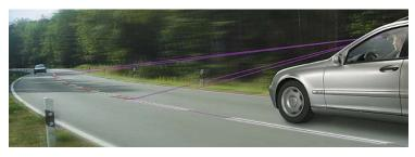
"... the system becomes an active lane keeping assistant as LKS, through an intervention in the steering. ... the LKS measures the vehicle position relative to the lane, but offers active support in keeping the vehicle to the lane. However, the driver always retains the driving initiative, meaning that although he can feel the recommended steering reaction as a gentle movement of the steering wheel, his own decision takes priority at all times..."
