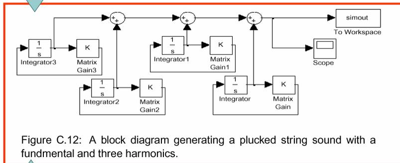
Figure C.12: A block diagram generating a plucked string sound with a fundamental and three harmonics.
