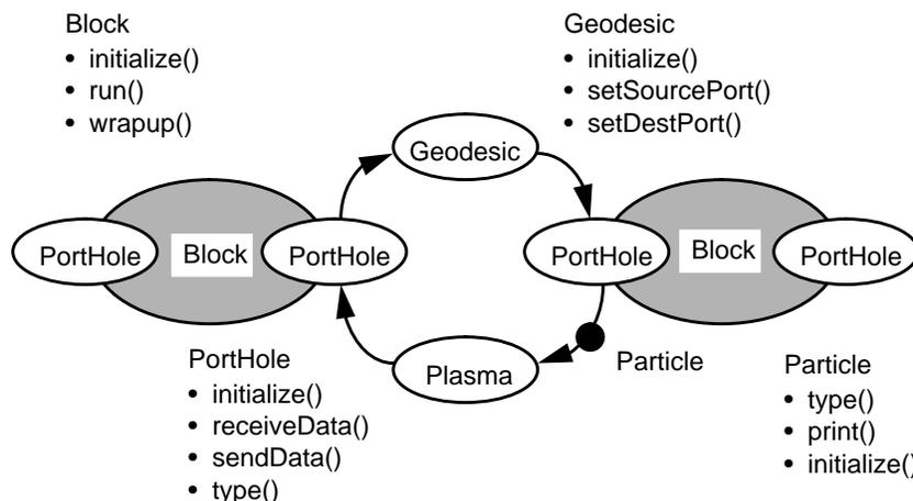
**Figure 3. Block objects in Ptolemy can send and receive data encapsulated in Particles through Portholes. Buffering and transport is handled by the Geodesic and garbage collection by the Plasma. Some methods are shown.**
