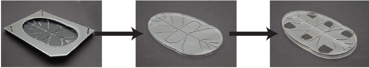
Figure 3.8: Images of the bottom shell mold, thermoformed bottom structural shell, and finished bottom shell after release cuts.
