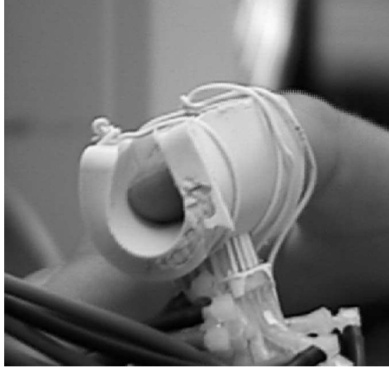
Figure 4.10: The tactile display attached to the finger.
