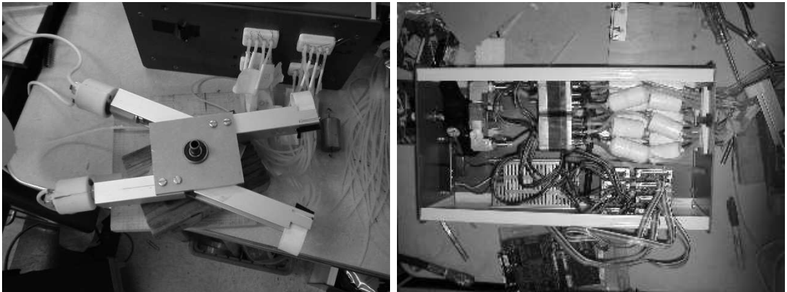
Figure 3.21: Pictures of the bidigital teletaction system along with the tactile display valves, low pass filters, and electronics.
