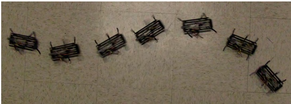
Figure 2.6: DASH can warp its body kinematics, changing its leg stroke, and inducing a turn. Figure courtesy of Paul Birkmeyer, used with permission.
