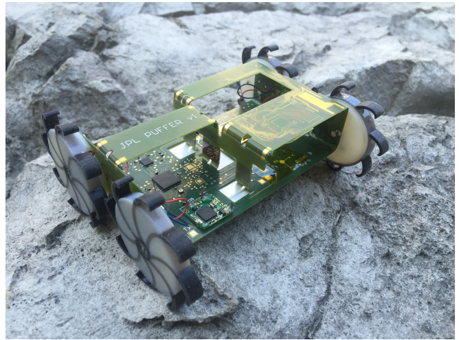
Fig. 4. First complete rigid-flex PUFFER prototype, built with PCB from second rigid-flex iteration. PCB was populated with a wirelessly-controlled motor driver circuit for driving the four independently-actuated wheels.
