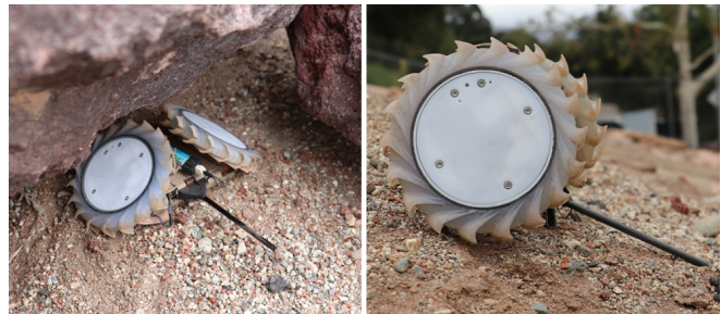
Fig. 11. Latest PUFFER prototype shown folded into a sprawled configuration to fit beneath a rock (left) and climbing a 20° slope (right).
