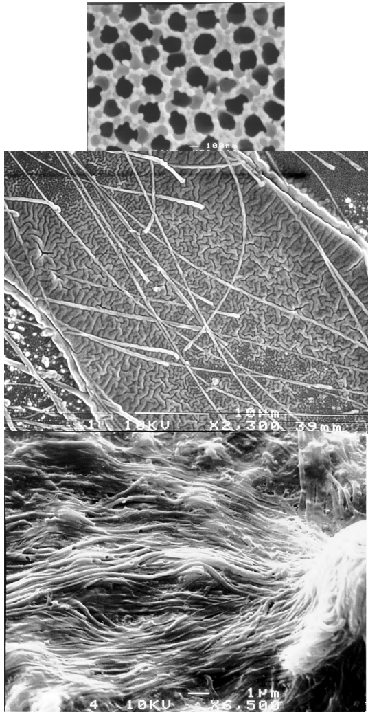
Fig. 6. SEM micrographs of (a) porous alumina membrane top-view (uppermost), (b) molded polyamide nano-hairs (middle), (c) molded silicone rubber nano-hairs (lowermost).
