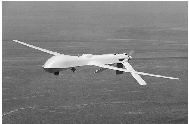
Fig. 1. The Predator Medium Altitude Long Endurance UAV (photo courtesy of US Department of Defense).
