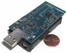
Figure 3: Telos ultra low power mote with IEEE. 802.15.4 wireless transceiver.
