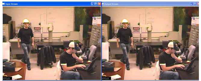
Fig. 3. Sample image frame input on left image, with output regions overlaid on right image. This sample illustrates where the intense light induced a specularity, causing the classifier to lose track of the hat.
