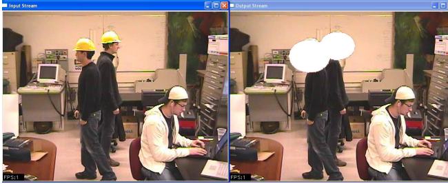
Fig. 5. Sample image frame input on left image, with output regions overlaid on right image. This sample illustrates tracking after a crossing (one frame after Figure 4), showing how the system successfully creates a second filter to best model the current scene.
