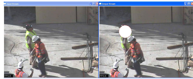
Fig. 7. Sample image frame input on left image, with output regions overlaid on right image. This sample illustrates how Particle Filtering overcomes partial occlusions, yielding a single, large ellipse.
