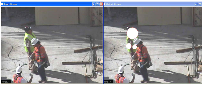
Fig. 6. Sample image frame input on left image, with output regions overlaid on right image. This sample illustrates how without Particle Filtering, partial occlusions segment the visual marker, resulting in multiple small ellipses.
