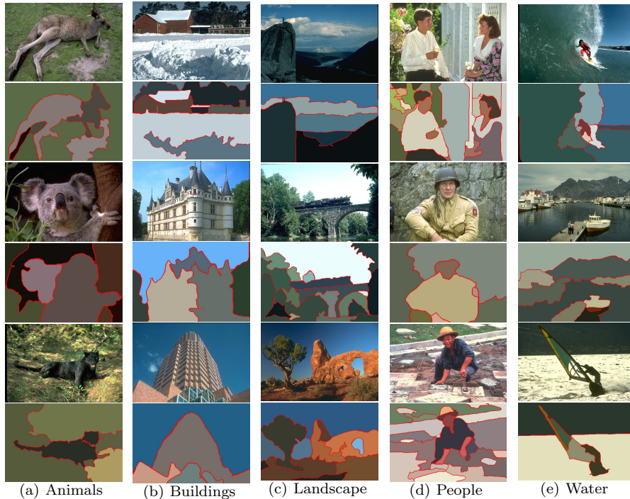
Fig. 8 Representative segmentation results (in color) of the TBES algorithm on various image categories from BSD. For each image pair, the top is the original input image, and the bottom is the segmentation result where each texture region is rendered by its mean color. The distortion \varepsilon was chosen adaptively to optimize PRI.
