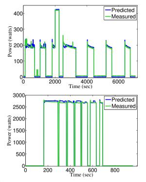
Figure 3: Actual and estimated electricity consumption of refrigerator (top) and washer-dryer (bottom) for House 1 using our proposed framework.
