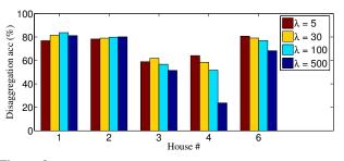
Figure 2: Effect of the regularization parameter  $\lambda$  on the disaggregation accuracy of our proposed algorithm for houses in the REDD dataset.
