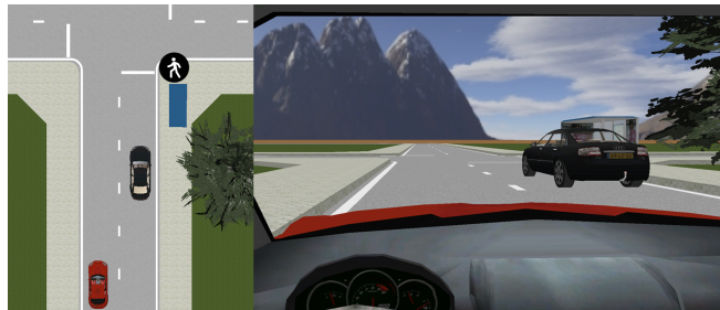
Fig. 1: Motivating example of occluded pedestrian. (Left) Topview showing the red ego vehicle, the black car causing occlusion, and the hidden pedestrian. We model the actions of the black car as sensor inputs. (Right) Viewpoint from the red car (ego vehicle), showing that the pedestrian is occluded.
