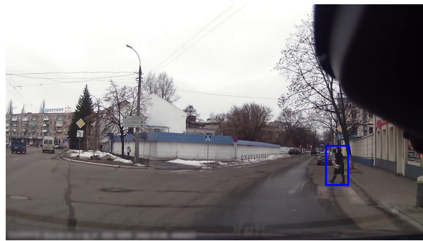
Fig. 6: Example image from JAAD Dataset with the pedestrian in a labeled blue bounding box [21].
