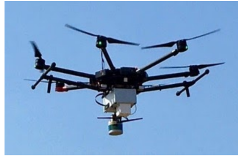
Fig. 2. Our sUAS is a DJI Matrice M600 that carries a LAMP sensor. In the image, the LAMP system can be seen underneath the sUAS and includes a LiDAR puck. The attached white box contains the radiation detection or imaging instrument.
