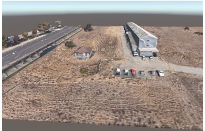
Fig. 5. Our VR interface consists of a baseline 3D mesh of the real world environment to orient the user in the virtual environment. The baseline mesh can be scaled or translated with arm gestures, allowing the user to navigate it while remaining stationary in the real world. Parked vehicles in this mesh may be used as a scale reference.
