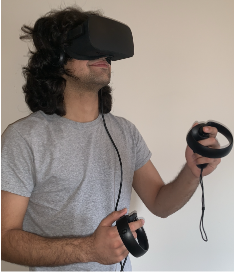
Fig. 4. A user can equip a VR headset and control the sUAS with VR controllers.
