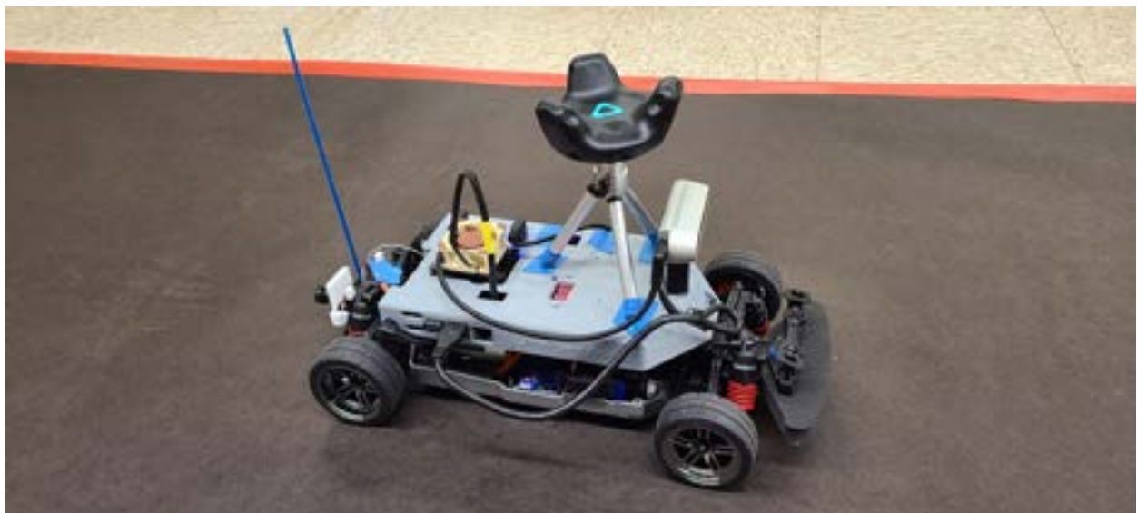
Figure 2.2: Original ROAR vehicle design with Vive Tracker
