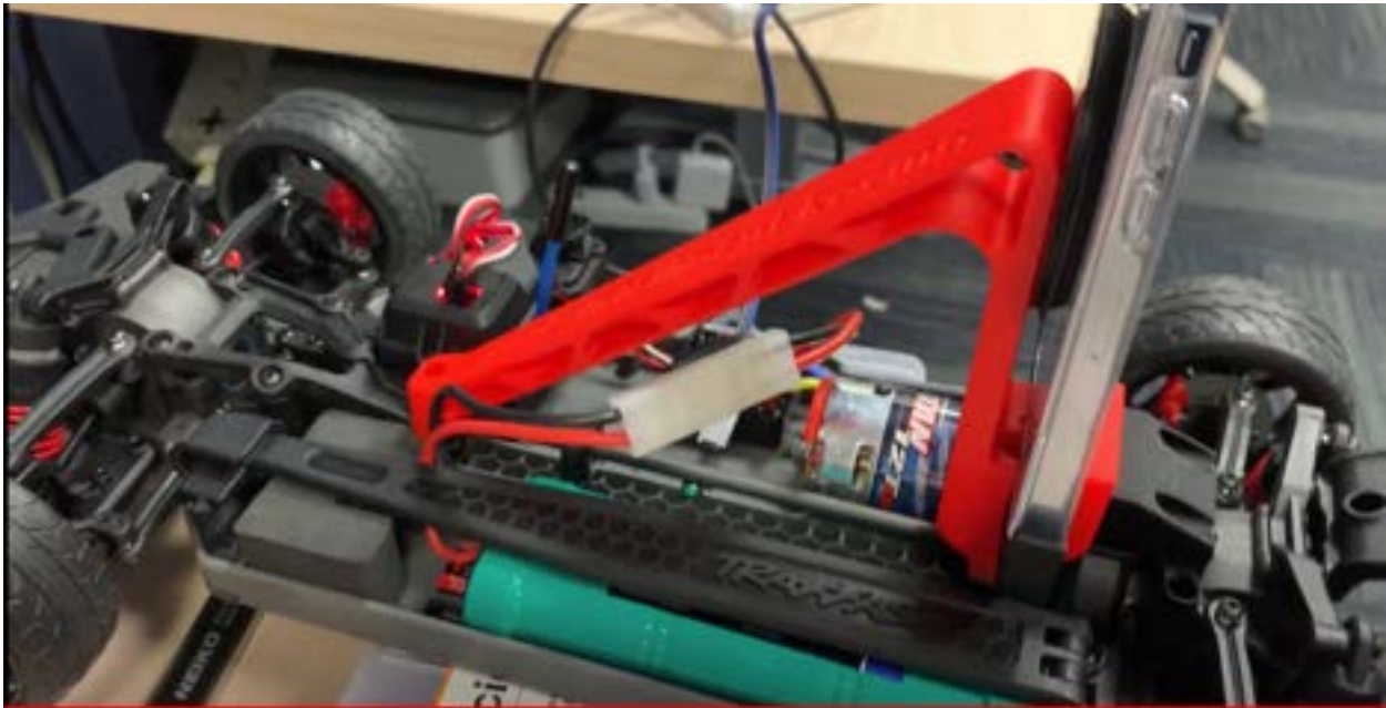
Figure 2.7: New iPhone mount with more structural integrity
