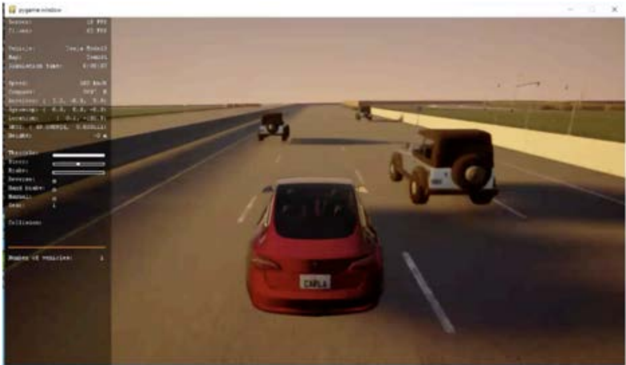
Figure 2.10: A screenshot of the CARLA simulator environment. The red car is controlled by a ROAR Python agent. Other vehicles can also be added to follow certain pre-programmed waypoints that share the same road. The simulator can also generate common vehicle sensor data, which is not shown here.
