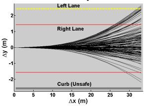
Figure 1: Example of an observed set of trajectories showing the change in lateral and longitudinal directions with respect to the center of the car at  $\Delta y=0$ .
