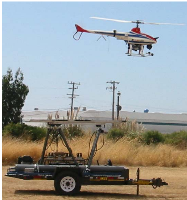
Figure 1: Berkeley UAV test-bed with on-board vision system: Yamaha R-50 helicopter with pan/tilt camera and computer box hovering above a landing platform.
