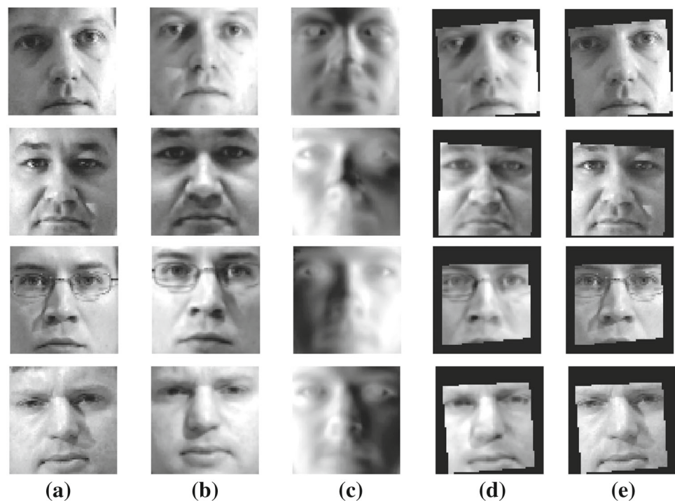
Fig. 4 Examples of warping a gallery image \tilde{a} and applying a mask \Omega on both the query image b and the warped gallery image \tilde{a} . a Query images b . b Gallery images a . c Illumination transfer information C\hat{y} . d Warped gallery images \tilde{a} under a mask \Omega . e Applying the same masks \Omega on b
