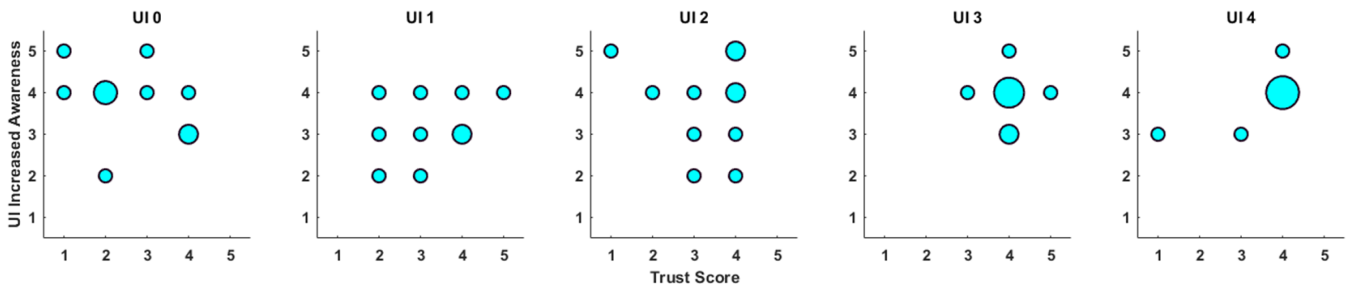
Fig. 7: The bubble plot shows the all subject responses to survey questions, where the size of the point indicates the number of identical responses. Each column corresponds to UI 0 through 4. The graph displays the Trust Score on the x-axis versus the agreement that the UI increased awareness on the y-axis.
