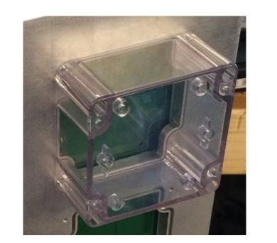
An off-the-shelf case seals modules to the waterproof sensing platform.
