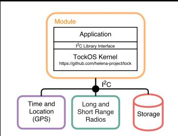
Onboard storage, communication, and energy management, plus software libraries for modules simplifies adding sensor modules to the system.
