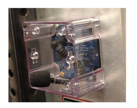
The case can be easily modified to accommodate different sensors.
