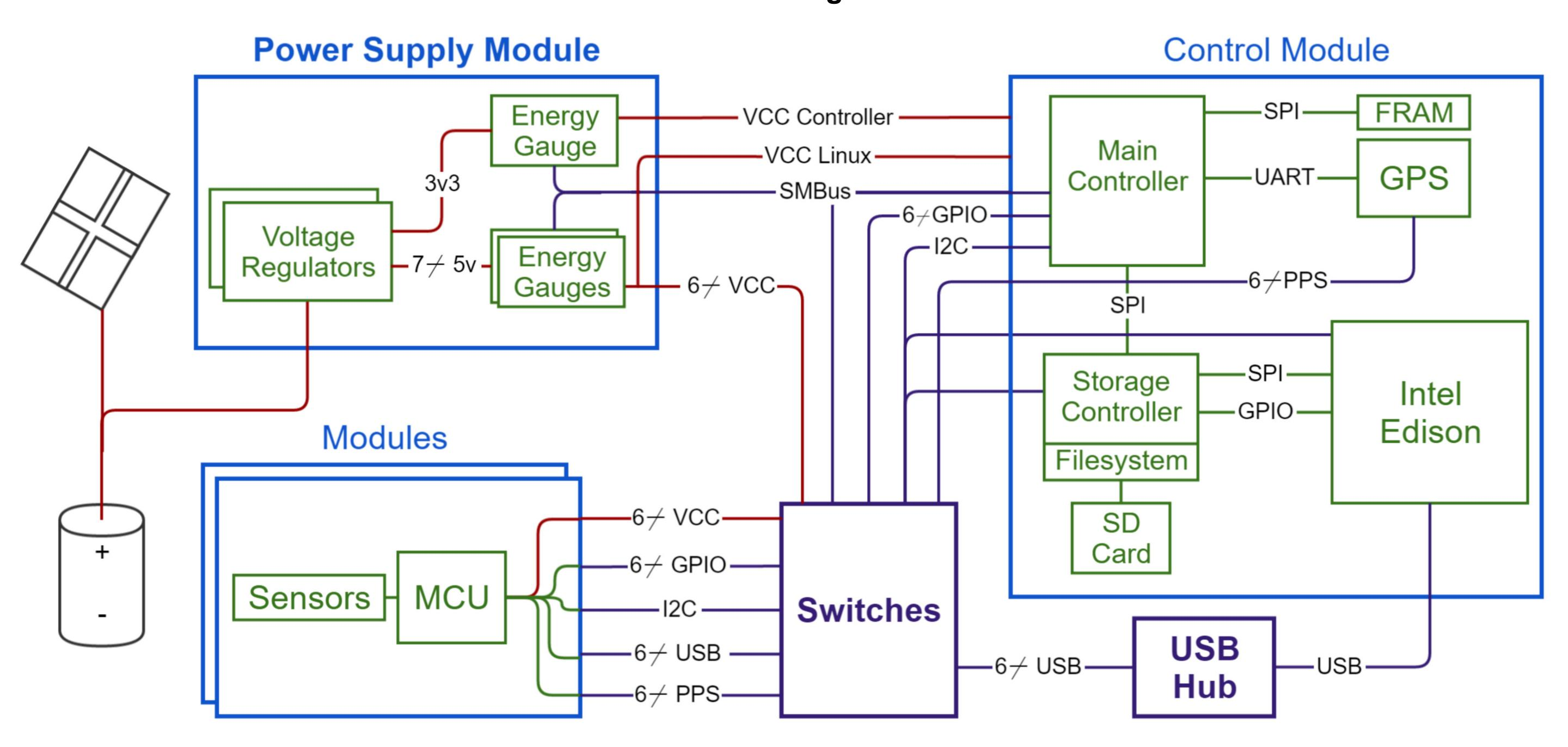
Interface. Sensor modules are added to the platform through a standard electrical and mechanical interface. The interface is designed to provide the necessary features we envision for modules.
