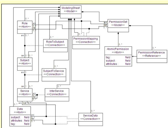
Permission mappings and actor interactions can be used to describe policies and interactions in Service Oriented Architecture.
