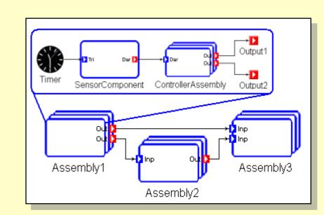
SMOLES is capable of capturing component structure, communication and component behavior. SMOLES does not allow the description of security properties of systems.
