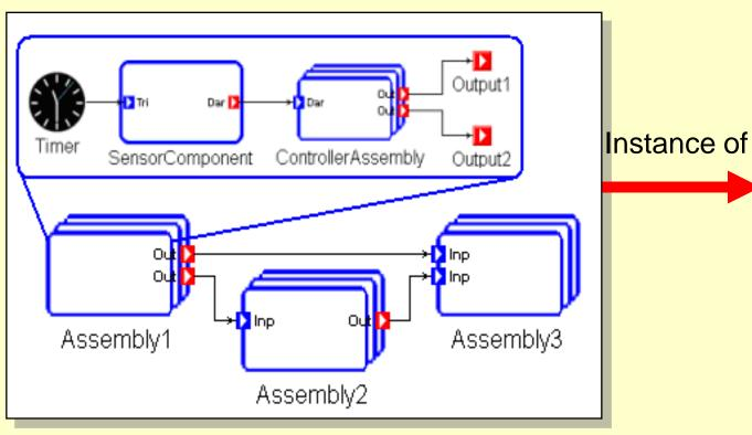
Model of an embedded system designed using the SMOLES modeling language.
