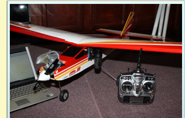
Aircraft with side-mounted camera, manual-control radio, and reported GPS tracklog
