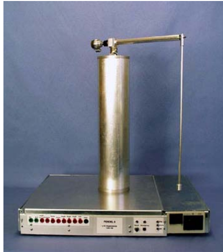
FIGURE 7.5 The Furuta inverted pendulum.
