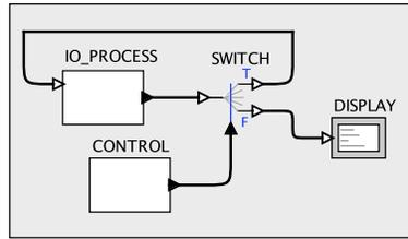
Figure 8: A program that has an infinite execution, but no bounded infinite execution. The CONTROL process is able to send messages to the SWITCH, but the SWITCH is unable to receive them because it is deadlocked with the IO\_PROCESS. If the CONTROL process can execute forever, sending control messages, then memory will overflow.
