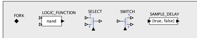
Figure 9: Five processes that, together with a boolean message data type, when connected in a KPN, provide a Turing-complete model of computation.
