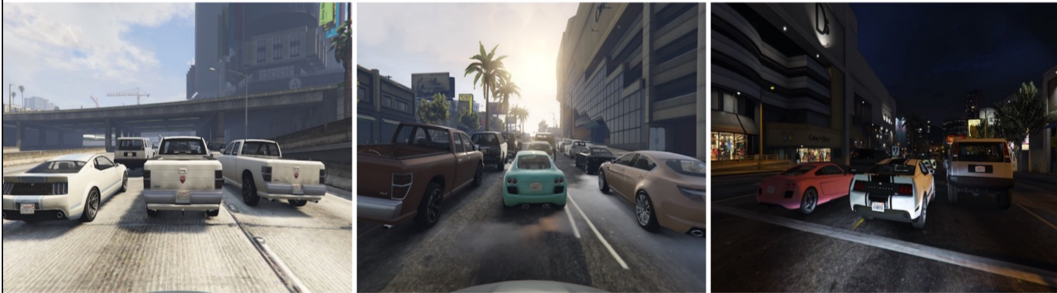
Figure 1: Three scenes generated from a single ~20-line SCENIC scenario representing bumper-to-bumper traffic.
