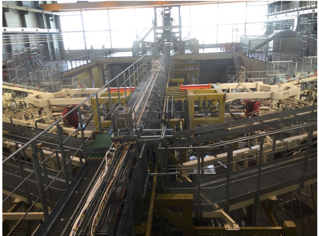
“Iron wing” model of an Airbus A350.
