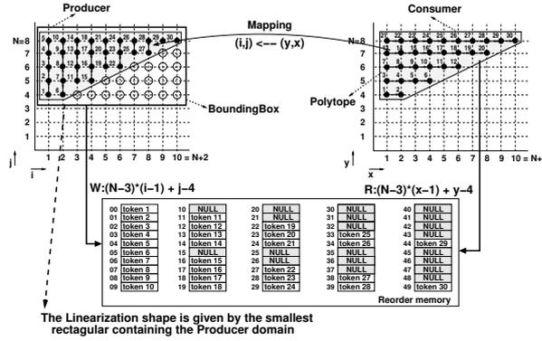
Fig. 4. The Linear realization of the reorder memory
