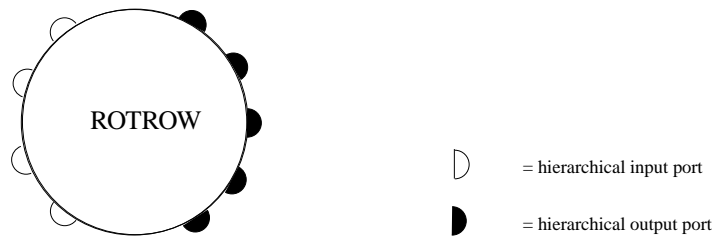
Figure 10.1. Segment node 'ROTROW' with its (hierarchical) ports, which are sets of ports.
